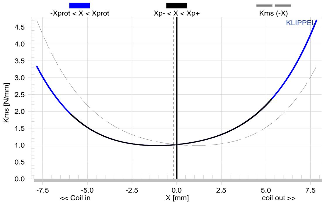
The  $K_{ms}(x)$  symmetry is not quite a perfect in this sample however a spider geometry change will improve this in production units. Still, the total asymmetry on this sample is only 1.5mm.
