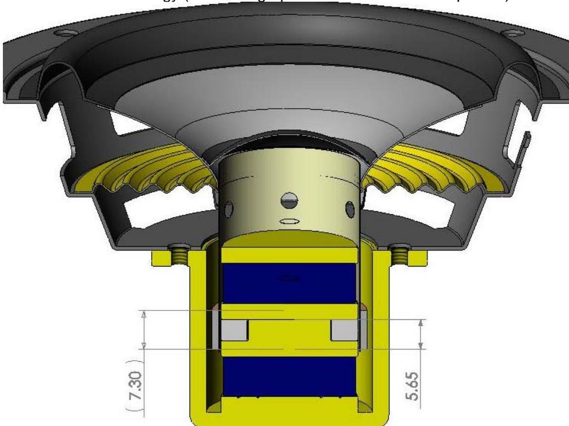
The physical  $X_{max}$  for an MMAG motor is calculated by:  $(WH - \text{Gap space}) / 2 + \text{Gap}$ . For this speaker the gap space is 4mm and we know the coil is 7.3mm so
