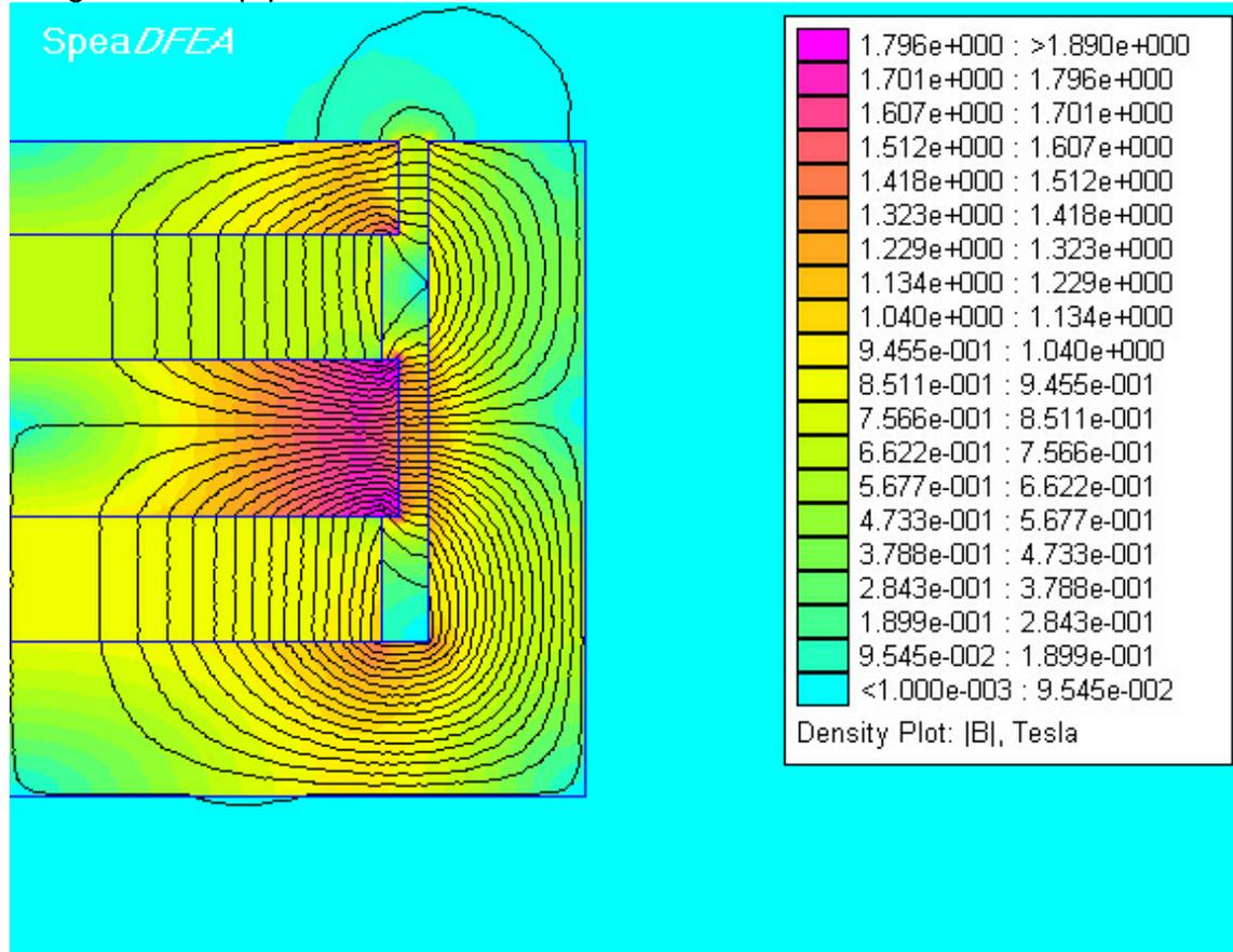
Using SpeaDFEA we get a BL of 7.75 and a coil Mmd of 1.73 for an efficiency ratio of 4.47.
