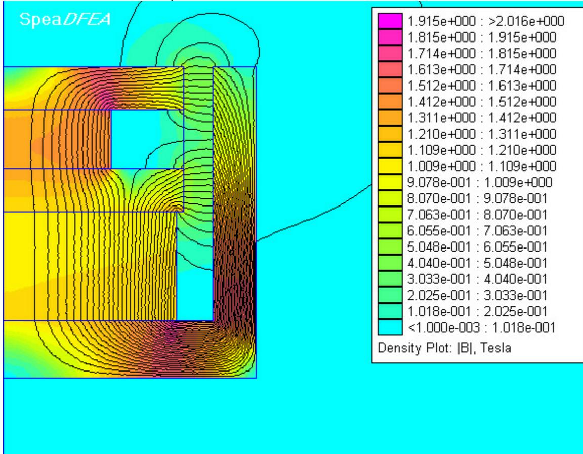
Note that there is an aluminum ring between the two gaps. This is another big advantage of MMAG; you can place a shorting ring right next to the voice coil – more about this in part 3.
