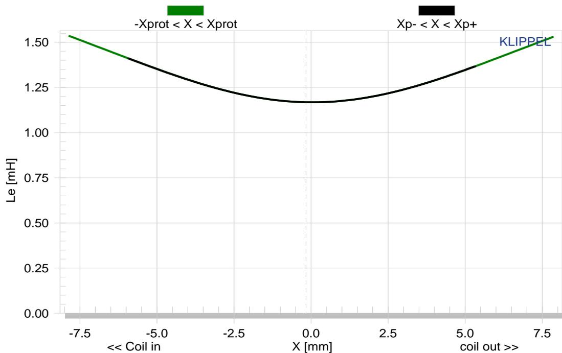
The non-linear inductance created by this motor system is virtually unique in speaker designs. Putting a shorting ring in the center of the virtual gap creates almost perfect symmetry, very low inductance and very low eddy currents in the steel parts. Klippel has shown that non-linear inductance is the most objectionable of the three non-linear components. The LRRP/MMAG motor reduces this component below the audible range even at maximum excursion.
