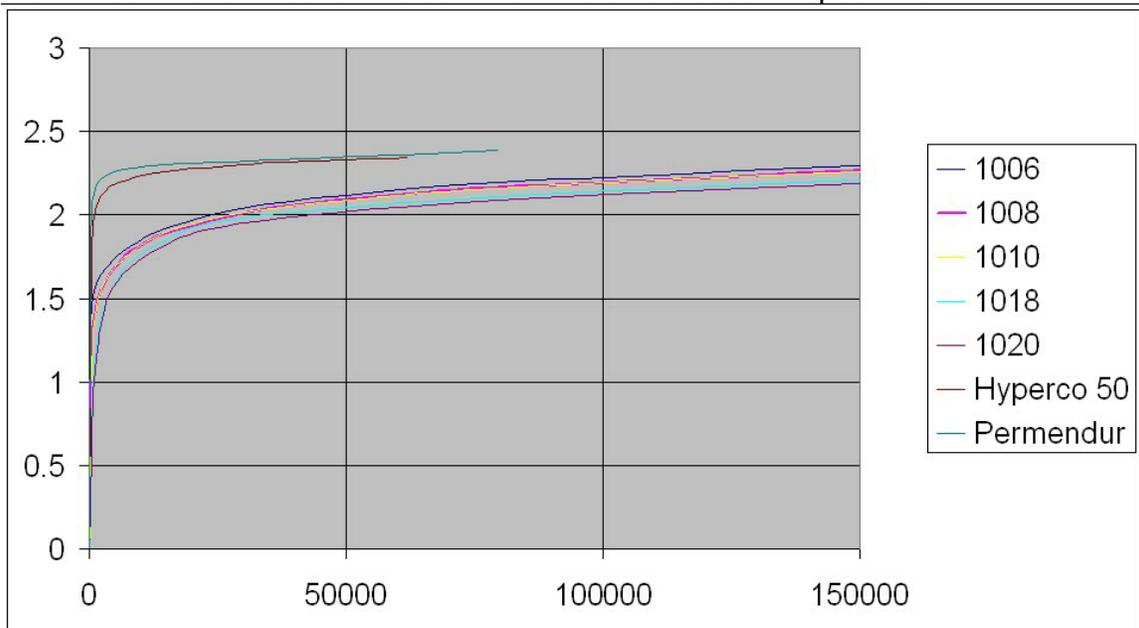
The sharp slope on the left side of the curves is the linear region and the flat section on the right shows where the material has reached saturation and can not pass any more flux. The transition point between these two slopes is called
