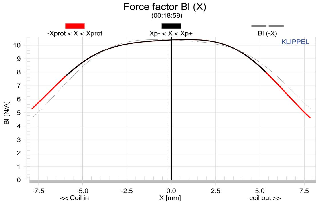
Note the symmetry is nearly perfect. This is a good example of balancing the gaps in an MMAG motor (which is actually quite easy).
